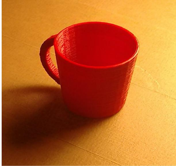
To do this, we can make the radius of the top of the cylinders greater than the radius at the bottom.
